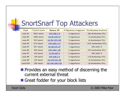
In using SnortSnarf as a quick, pull based "summarizer" or snort reporting tool, an analyst can quickly drill down to some of the more important events on the network.
