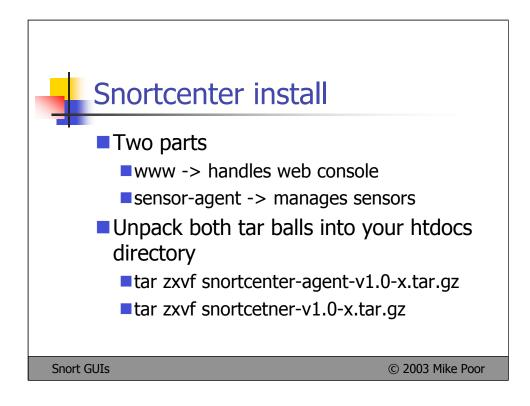
The install comes with two parts. A web console section, and a sensor management section. If you are installing both parts on one machine, untar the packages in your htdocs directory of your webserver.
