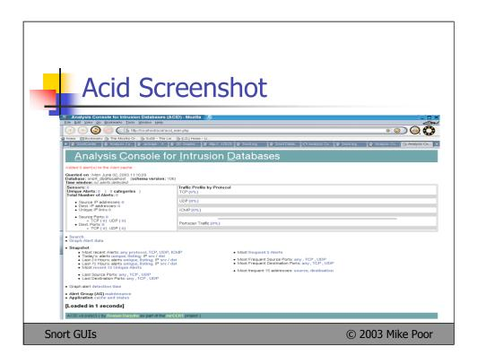
Acid's main screen. Acid allows one to query a database of event information for specific data. One can query the db for all events from a range of time, from a specific IP address, or specific event and so on.
